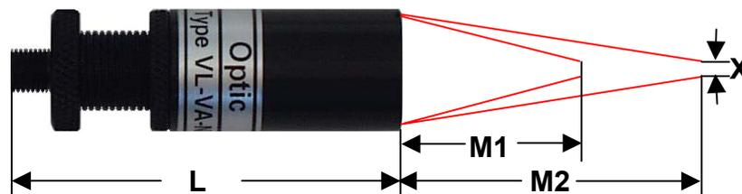
target size X:  $\frac{\text{focusing distance M mm}}{\text{distance ratio D}}$  par ex.  $\frac{M = 150\text{mm}}{D = 75} = 2,00 \text{ mm } \varnothing$
